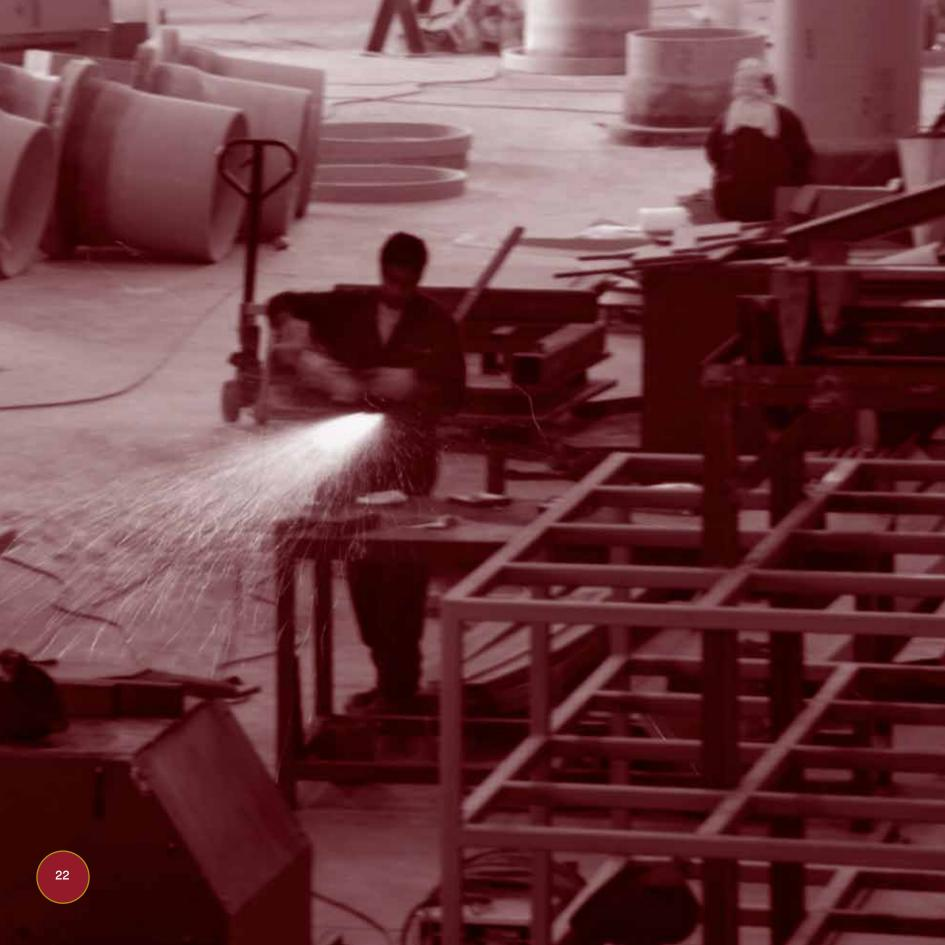
The method of fabrication of all GRP fittings is essentially the same. Pipes, after plant hydro-testing, are cut to the required dimensions. Pipe sections are then joined together by lamination. The thickness and width of the lamination is designed to exceed pipe performance.
